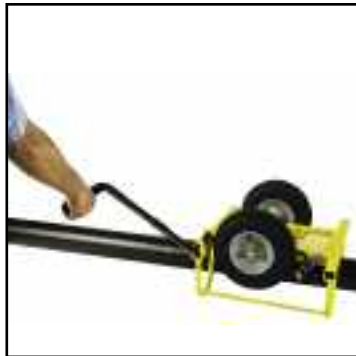
1 use ratchet to secure Cricket to pipe
