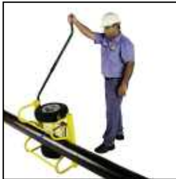
2 use handle to flip Cricket & pipe
