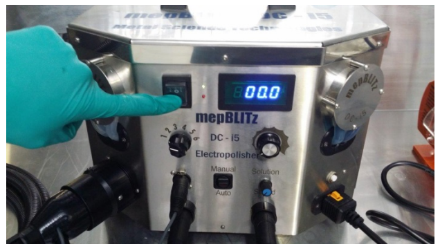
ON OFF switch turned ON
