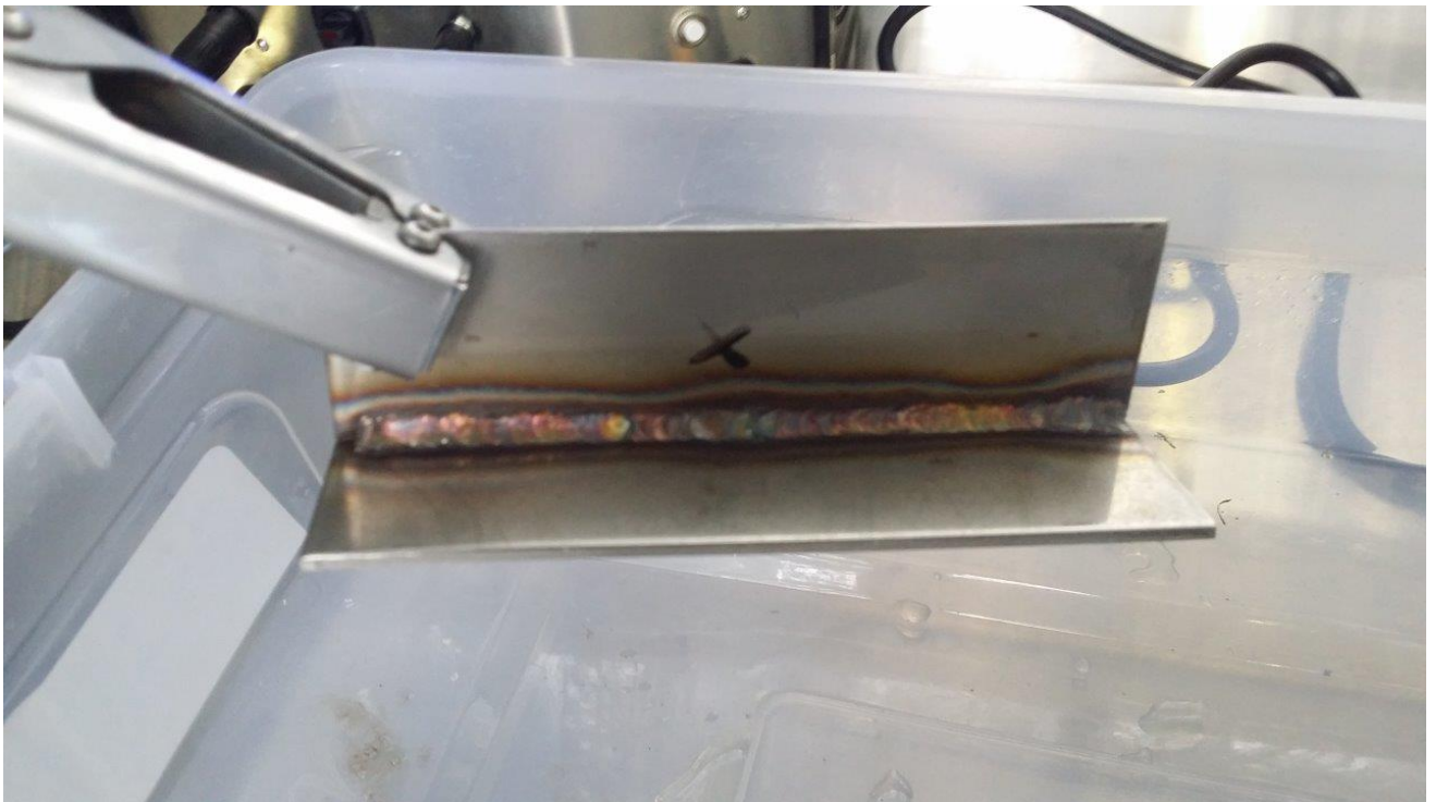
Clamp attached to the work piece ready to be cleaned
