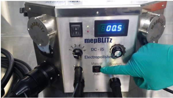
Auto/Manual button in the manual position
