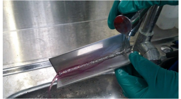
Running water removing neutraliser from work piece
