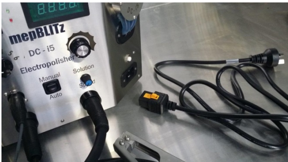
Input power cable ready to be attached
