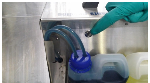
Release momentary switch once coolant has circulated
