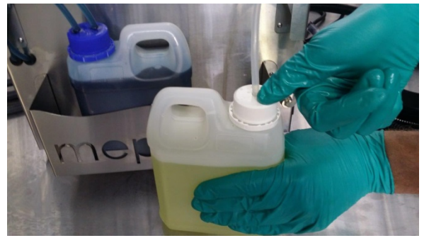
Hold thumb over hole in the lid and squeeze bottle to push solution
