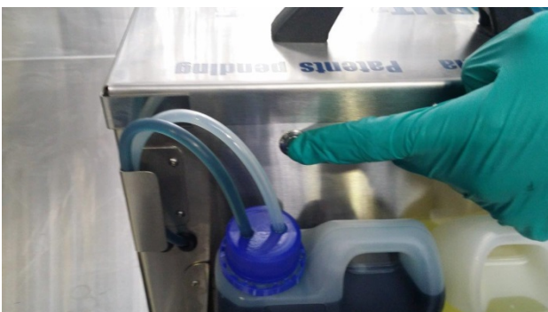
Hold momentary switch until coolant reaches the pump on the front of machine
