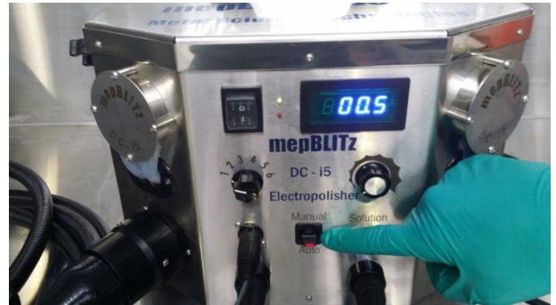
Auto/Manual button switch to the auto position
