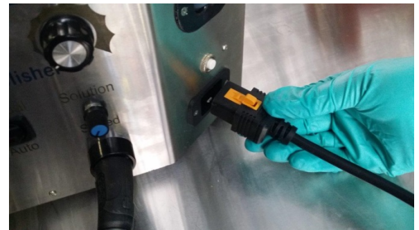
Input power cable being attached
