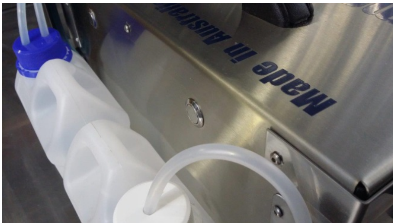
Stainless steel switch flush, solution pump will run forwards
