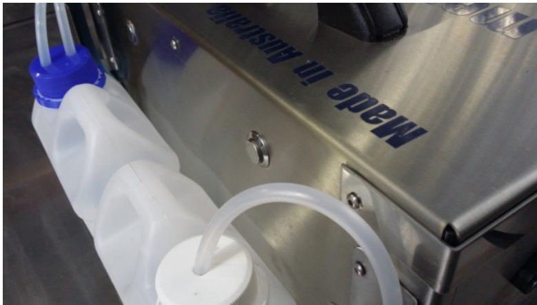
Stainless steel switch raised, solution pump will run in reverse
