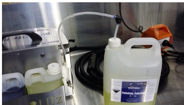
Tube extension tapped into 5lt bottle
