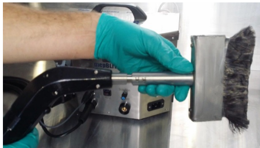
Slide M120 brush onto torch
