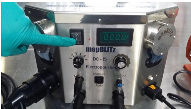
ON OFF switch in the OFF position
