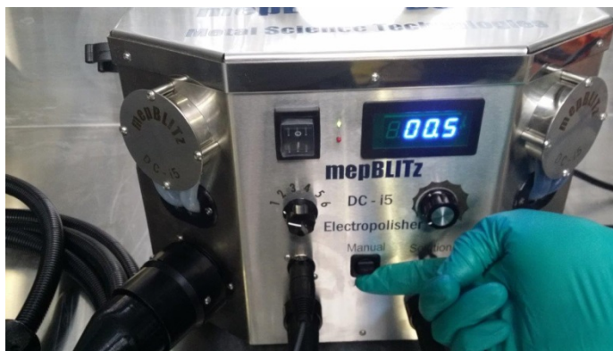
Auto/manual button back to the manual position
