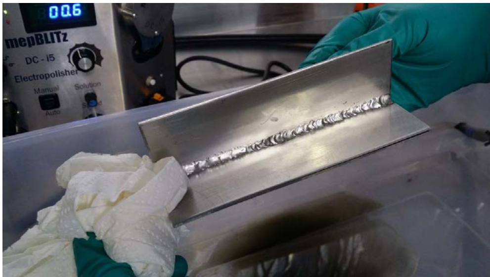
Cleaned weld piece being wiped down
