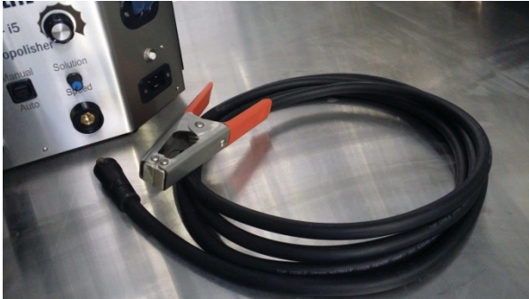
Earth Clamp ready to be attached
