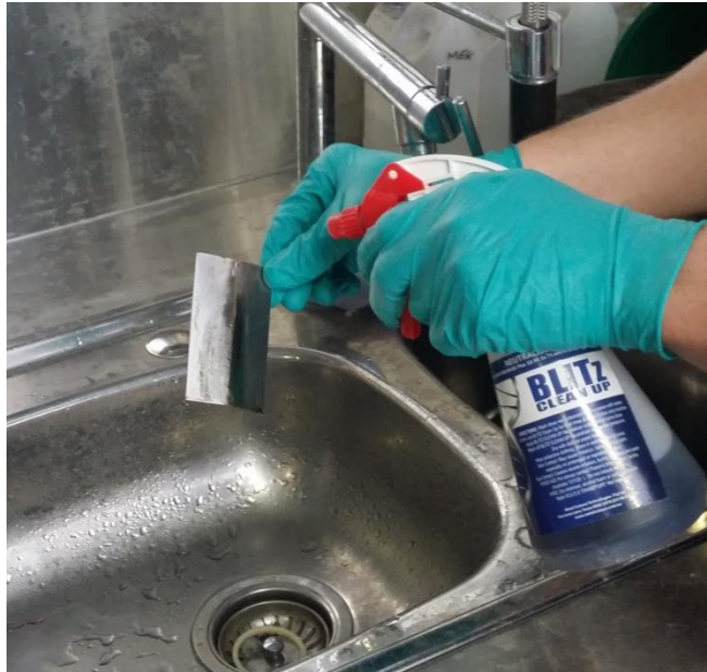
Neutraliser about to be sprayed onto cleaned weld
