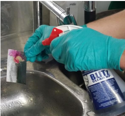
Neutraliser being sprayed onto cleaned weld
