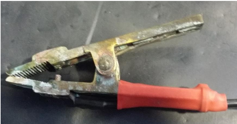
Un-cleaned Clamp with corrosion
