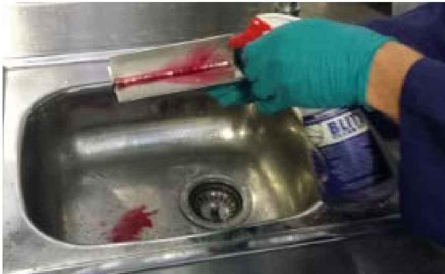
Neutralizer being sprayed onto cleaned weld
