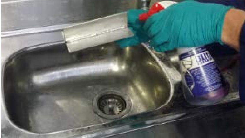
Neutralizer about to be sprayed onto cleaned weld
