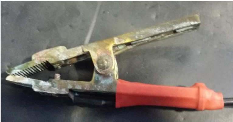
Un-cleaned Clamp with corrosion
