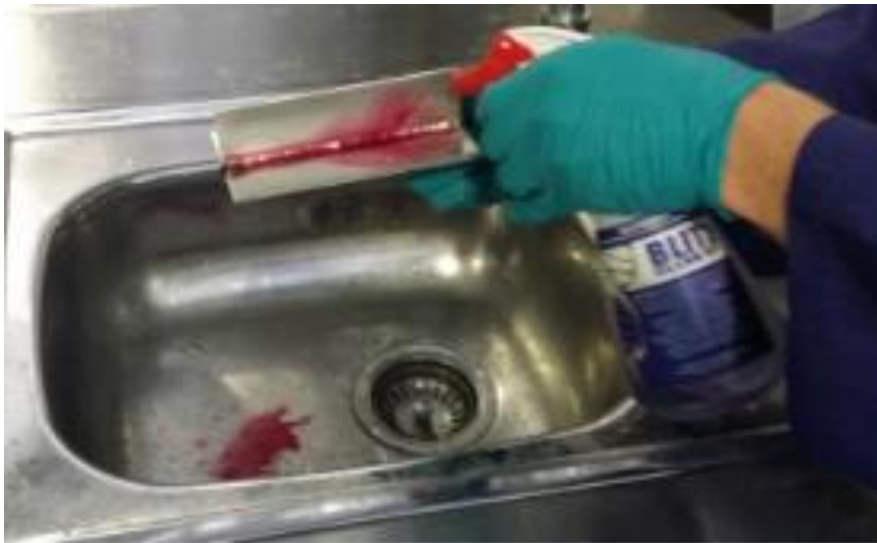
Neutralizer being sprayed onto cleaned weld
