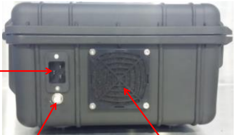
Primary Circuit Breaker
