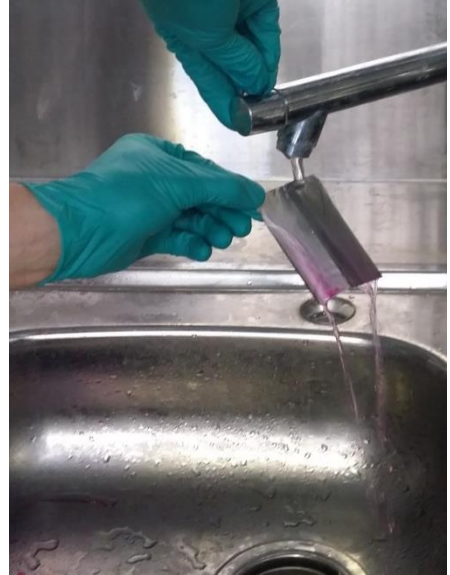
Running water removing neutraliser from work piece
