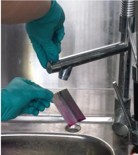
Remove residual neutraliser with running water
