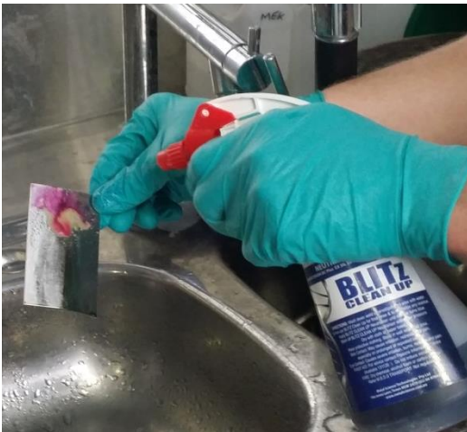
Neutraliser being sprayed onto cleaned weld
