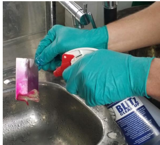
Neutraliser being sprayed onto cleaned weld
