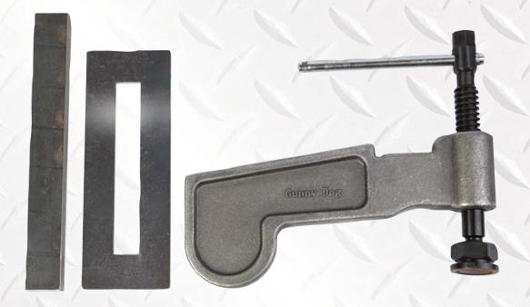
Non- welded fitting aid assists in the make-up and gapping of vertical seams, deck seams, knuckles, and other plate joints that typically require the use of dogs, wedges, fishtail jacks, or other weld-on fitting aids.
