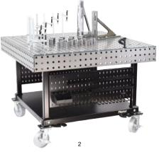
Welding table 122 x 122 x 89cm (I x w h), with 1.27cm top supported by 0.95 x 12.7cm struts every 40.6cm, Flextur tool board panels, a full bottom shelf, casters, and a 907kgs. capacity. Surface flatness is +/- 0.0381cm over the 32 square feet area.
