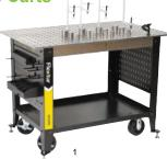
Mobile welding cart with 42 piece fixture & tool board accessory kit capable of supporting and transporting 793kgs.
